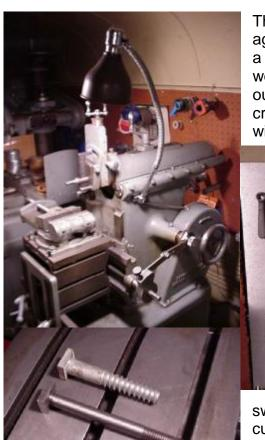
The lamp came from another machine and I attached it years ago (before I realized that drilling and tapping into a machine is a "no-no.") The 2 mount screws were drilled in a spot that would not harm the machine and for all practical purposes are out of site. It is a great aid in seeing those tiny numbers on the cross feed dial! The lamp can also swivel to the right and assist with the Alexander (think Deckel F1) mill.
