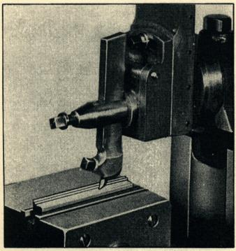
Fig. 4. Straight Cut on Flat Piece of Work.
