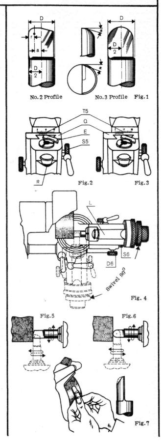
Where pointed cutters are concerned, both the included angle of the point and the back rake angle are produced in one operation (see Fig. 1). The back rake angle should be selected to suit the material to be cut (see Sheet 2109).
