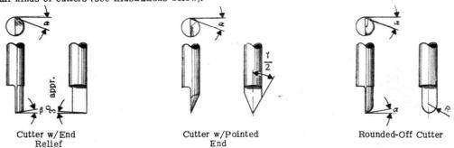
Angle  $\beta$  applies for end relieved cutters only. Cutters having an angle  $\alpha$  of less than 20° should be relief ground at between 25° and 30° (see special instructions).
