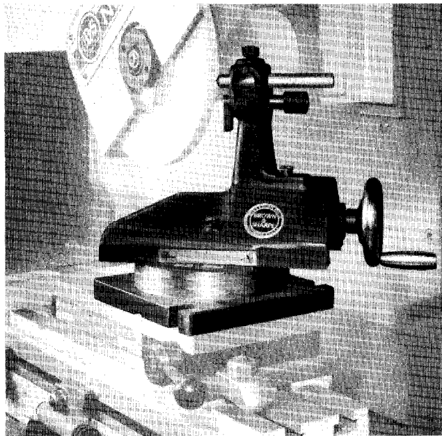
Fig. 24. Shaping a radial contour with Radius and Angle Wheel Truing Attachment. The slide is clamped at the required radius, the diamond tool is set by the gage just below it and the slide is swiveled to form the wheel.
