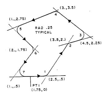
N5G0X1.75Y0Z0; MOVE TO PT1 N10G1X1.75Y.5F20.; FEED TO WORK N15G23X2.5Y.5R.25; DO FILLET 1 DO FILLET 2 DO FILLET 3 N20G22X3.5Y2.OR.25; N25G23X4.5Y2.25R.25; DO FILLET 4 N30G23X3.0Y3.5R.25; N35G23X1.0Y2.75R.25; DO FILLET 5 N40G22X2.Y1.75R.25; DO FILLET 6 N45G23X1.Y.5R.25; DO FILLET 7 N50G1X1.75Y.5; LINEAR TO EXIT PT
