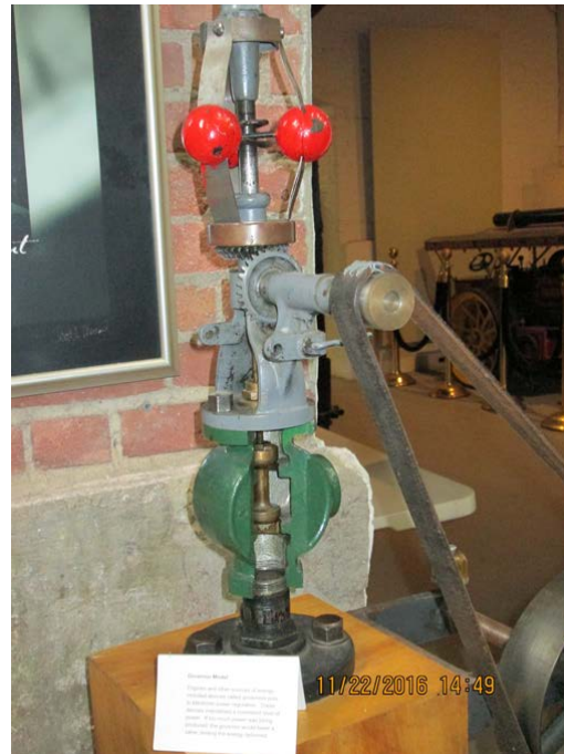
Figure 1: Steam Engine Throttle governor The belt turns the vertical shaft, which causes the red balls to rotate. Centrifugal force causes the balls to move outward, moving further outward as the speed increases. The pivot for the balls is anchored at the bottom, so the outward motion of the balls causes the vertical shaft to drop , which closes the valves in the green painted enclosure.
