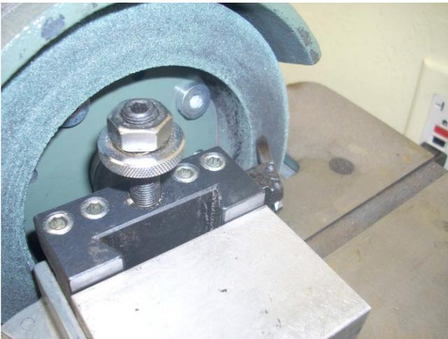
Here you can see me grinding the cutting edge used for turning. I am using a block behind my toolblock to set the angle with respect to the small slide angle support that came with the grinder. It took a little trial and error to figure out how far to stick out the HSS blank so the toolholder clears the wheel.
