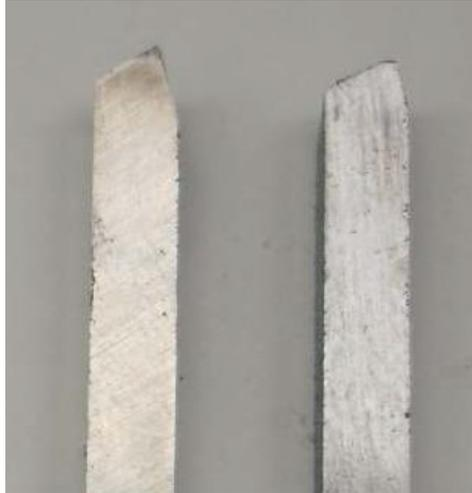
Here you can see the cutting edge used for facing. The one on the left is from Mr. Wimberley while the one on the right is mine.
