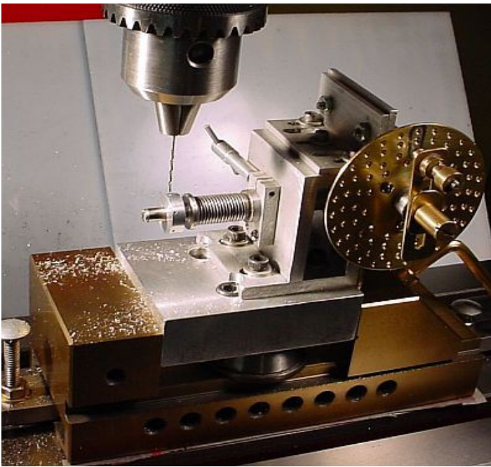
Drilling Radial Teeth
