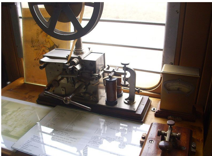
A Printing Electrical Telegraph Receiver, with Transmitter Key at Bottom Right
