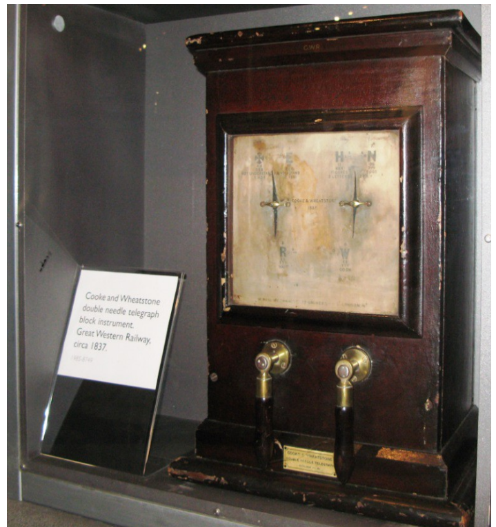
Cooke and Wheatstone Double-needle Telegraph Instrument of the Type used on the Great Western Railway
