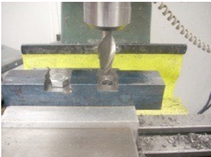
Milling for Bolt Heads Photo by R. G. Sparber
