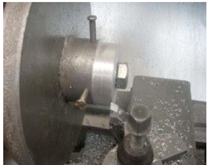
Cutting Hub Photo by R. G. Sparber
