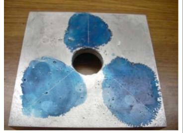
Without PinPhoto by R. G. SparberI removed the pin so the radial locations of the mounting<br/>bolts could be scribed.
