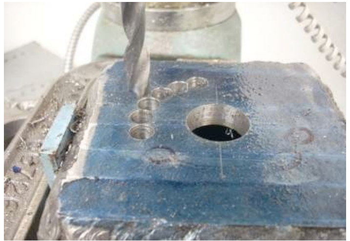
Chain Drilling Photo by R. G. Sparber
