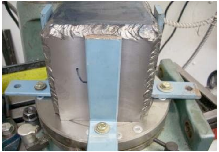
Brackets Holding Box Photo by R. G. Sparber
