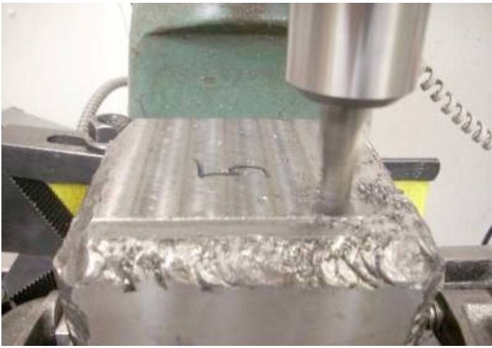
Milling End Plate Photo by R. G. Sparber
