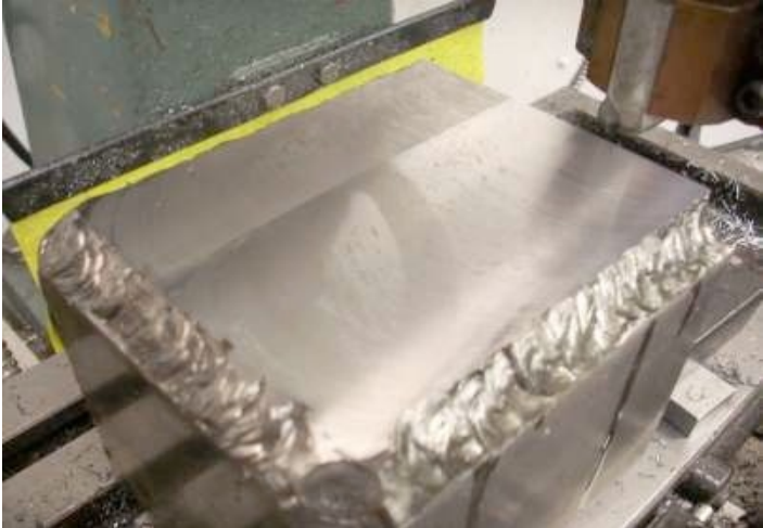
Shell Mill Face Photo by R. G. Sparber
