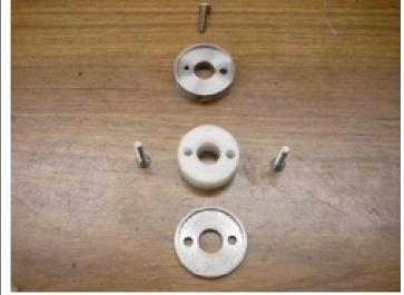
Dial Parts Photo by R. G. Sparber There is nothing special about this lathe work. The top and bottom are CRS. The recesses are 0.05" deep and cut with a boring bar. The plastic is Delrin®. The plastic scale is 0.005" thick so there is a 0.006" difference in radius between the plastic puck and the ID of the recesses. The puck was turned to exactly 1.000" diameter to match the scale which is 3.146" long (circumference = pi x diameter).
