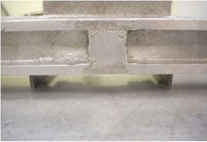
Casting on Parallels Photo by R. G. Sparber
