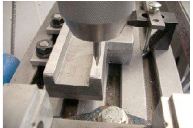
Locating Center of Pad Photo by R. G. Sparber
