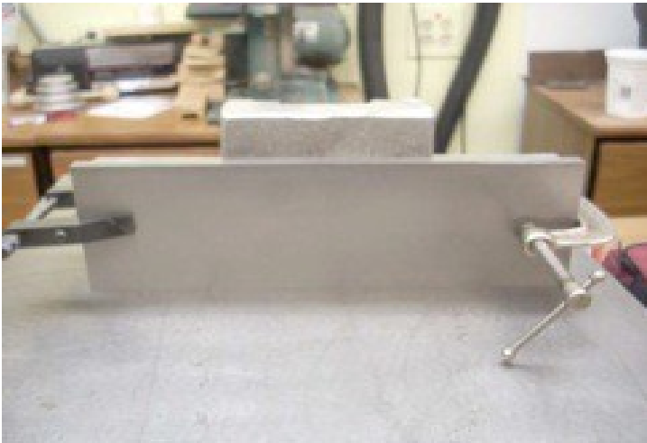
Centering Plate on Casting Photo by R. G. Sparber
