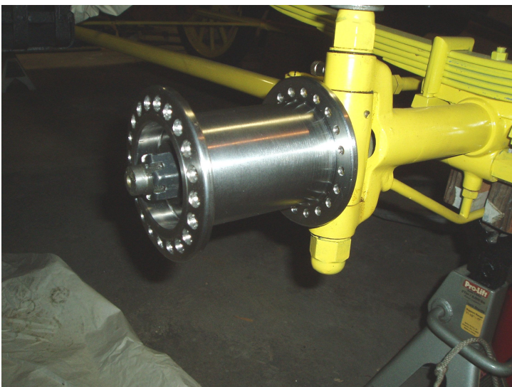
Finished Front Hub
