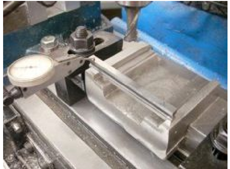
Checking Side to Side Photo by R. G. Sparber
