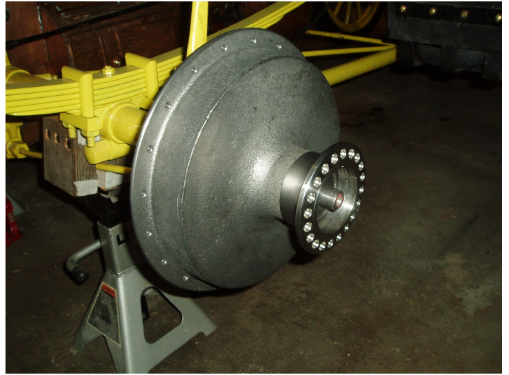
Finished Rear Hub
