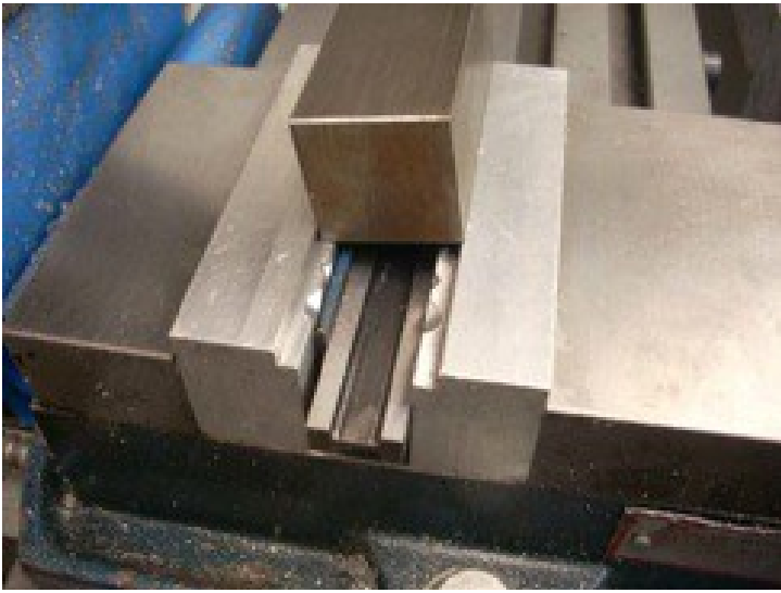
Recutting Soft Jaws Photo by R. G. Sparber
