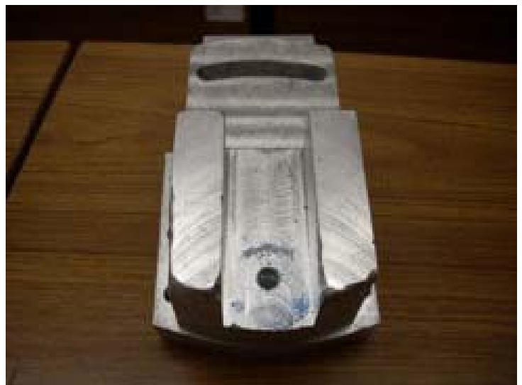
After More Surface Milling Photo by R. G. Sparber
