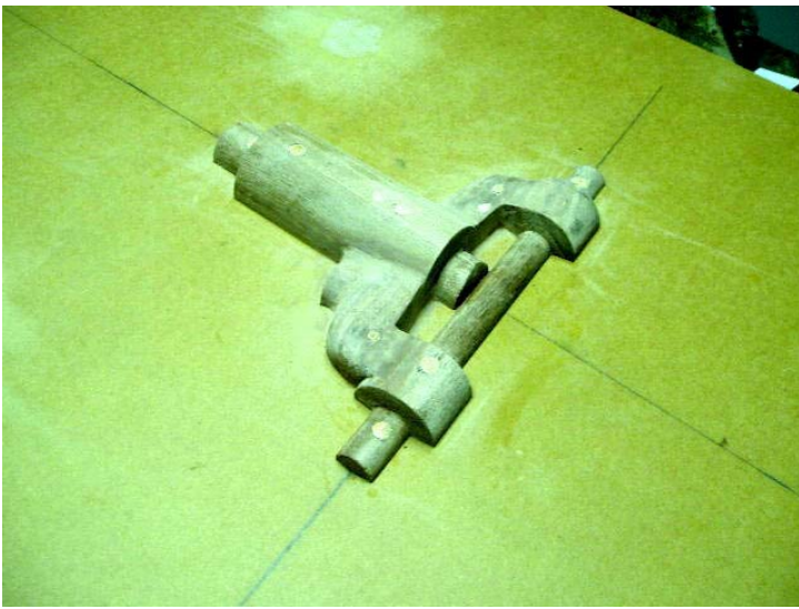
Match plate pattern with standard cores - Un-gated
