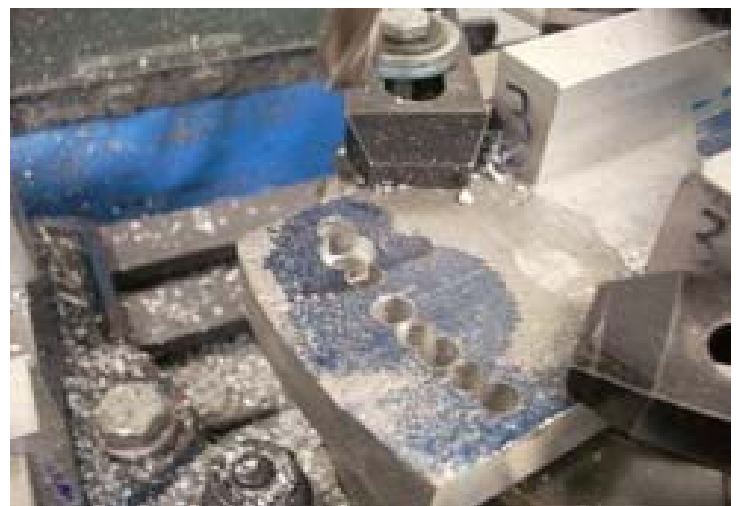
Milling Slot Photo by R. G. Sparber
