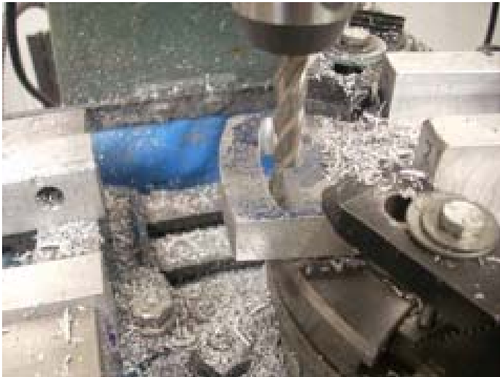
Side Milling Slot Photo by R. G. Sparber
