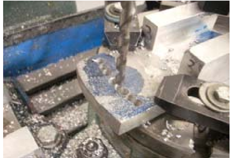
Chain Drilling Continues Photo by R. G. Sparber
