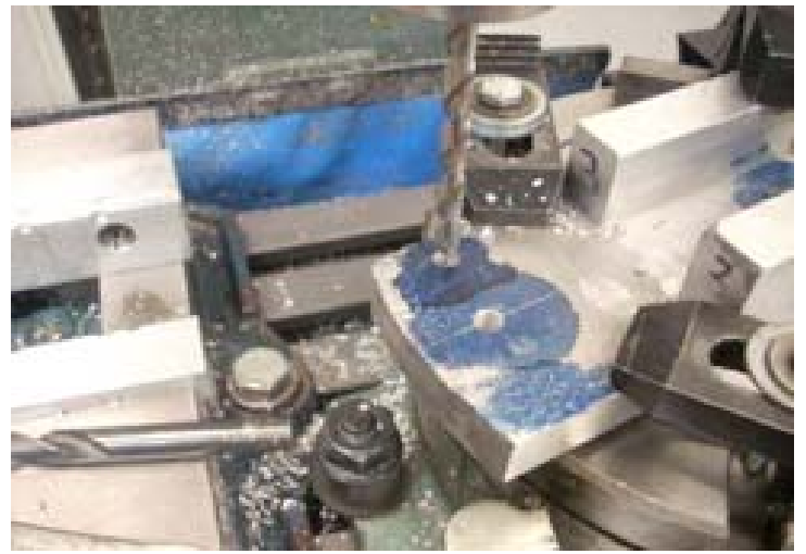
Chain Drilling Begins Photo by R. G. Sparber
