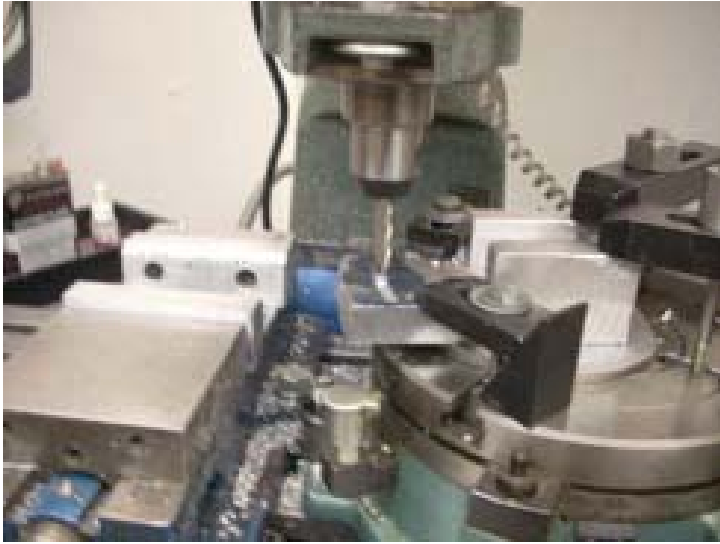
Really Milling Slot Photo by R. G. Sparber
