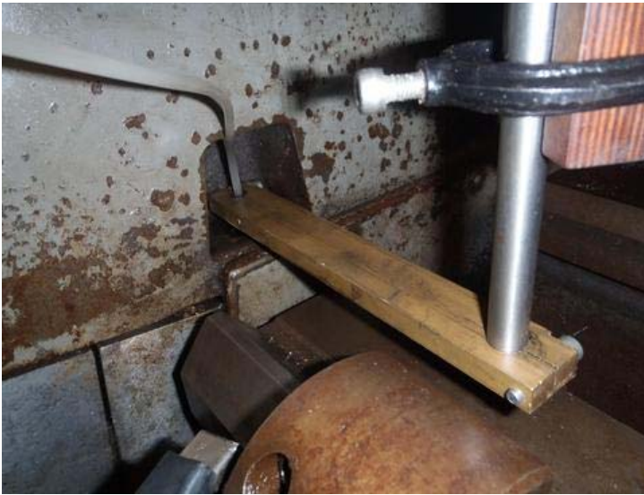
Here's the complete set up. The Servo head is conveniently mounted onto the lathe's toolpost and the electrode is on the end of the brass bar, within the lathe's headstock casting.
