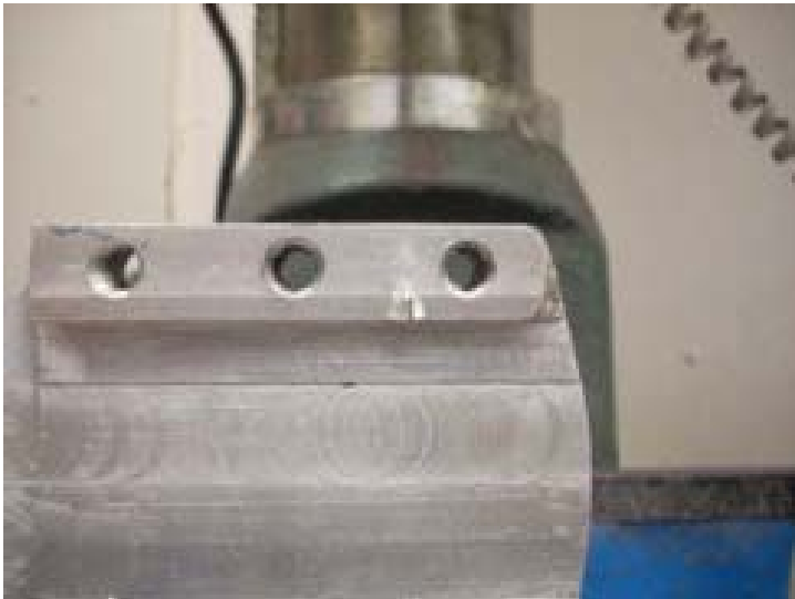
Gib Screw Break Out Photo by R. G. Sparber
