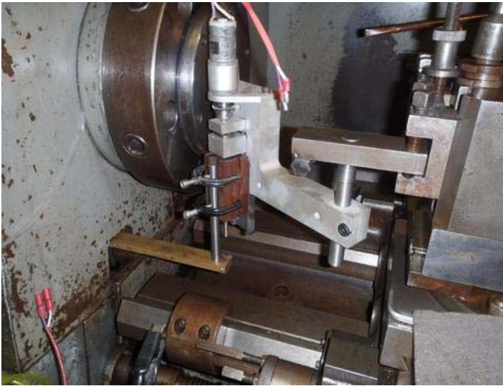
The tank, with pump, filters etc is on the headstock and supplies the centre flushing to the electrode. Most of the fluid is caught and reused. There's actually only a small flow once the electrode starts entering the work.
