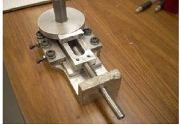
Down Feed Assembly Photo by R. G. Sparber Above we have the down feed almost done. The round bar sticking up, the disk, and the rectangular part with the slot in it make up the slide and was described earlier. Next, I will describe machining the L shaped casting, fitting the slide clamps, and fitting the previously turned drive screw.
