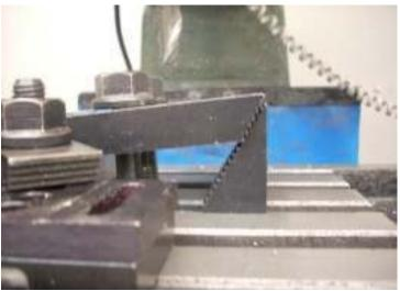
Hold Down Clamps Photo by R. G. Sparber On the right side are two hold down clamps that are raised slightly as you will also see below. The eccentric screws are first turned so the narrow part is facing the casting. Then the casting is pressed against these screws. Next the two hold down clamps are pressed against the casting. A quarter turn on the screws and the casting is pushed towards the clamps and down onto the support plate.
