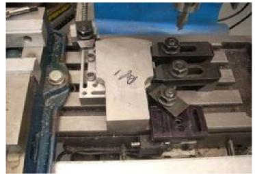
Mill Setup 2 Photo by R. G. Sparber My mill table is true and I have placed a support plate down that is of uniform thickness. As long as Reference 1 prime is firmly against the support plate, Reference 1 will be parallel to it.
