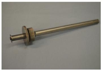
It's a 6" long gage marked "C. F. Richardson, Athol, MA." The Richardson family owned a small manufacturing firm notable mostly for the fact that it made the earliest version of LaRoy S. Starrett's highly innovative combination square during the first couple of years it was manufactured. C. F. Richardson made a variety of machinist's tools and other products, but it was never a large operation and ultimately Starrett bought them out in 1907.
