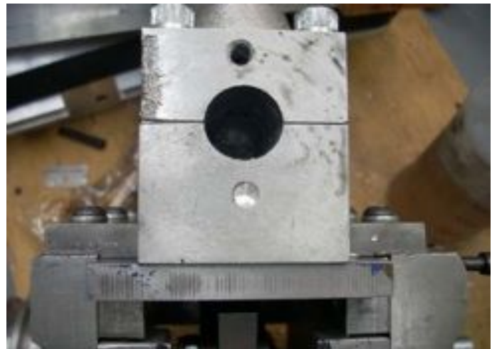
Clearance Drill Result - Photo by R. G. Sparber
