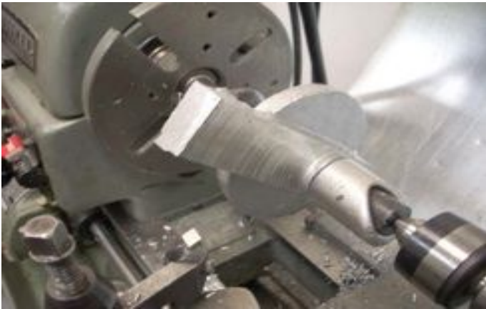
Facing Downfeed - Photo by R. G. Sparber
