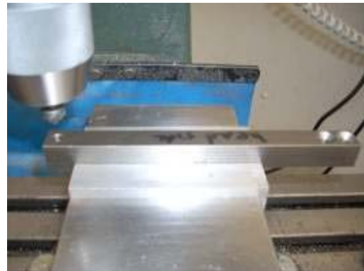
Countersinking Photo by R. G. Sparber
