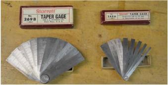
The A gage measures holes from  $\frac{1}{10}$  to  $\frac{1}{2}$  inch and the B gage goes from  $\frac{1}{2}$  inch to 1 inch, with both gages being graduated in increments of 0.001". These gages are small, only  $2\frac{3}{4}$ " long. As far as I know, they are still in Starrett's catalog.
