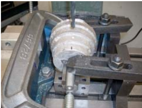
Mill Setup for Set Screw Photo by R. G. Sparber
