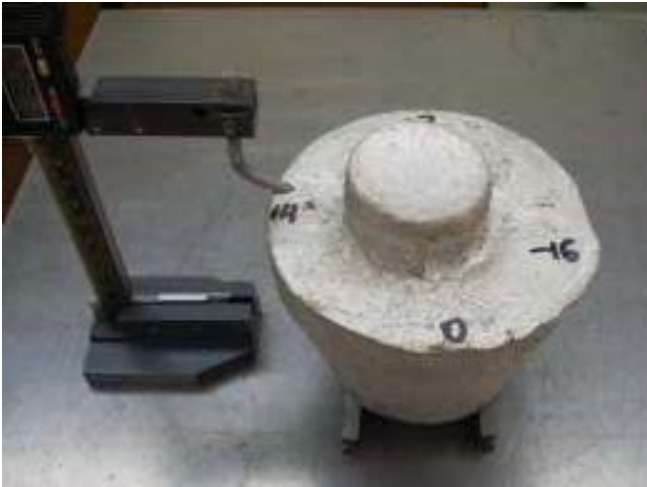
Marking High & Low Photo by R. G. Sparber
