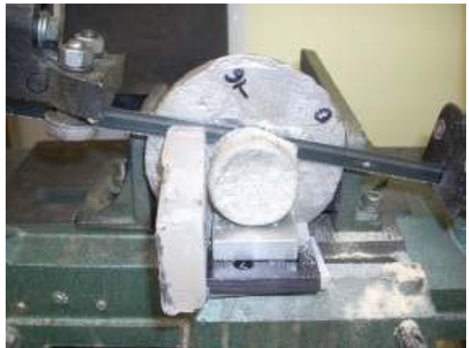
Cutting with Wax Photo by R. G. Sparber
