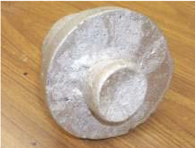
Casting with Sprue Photo by R. G. Sparber
