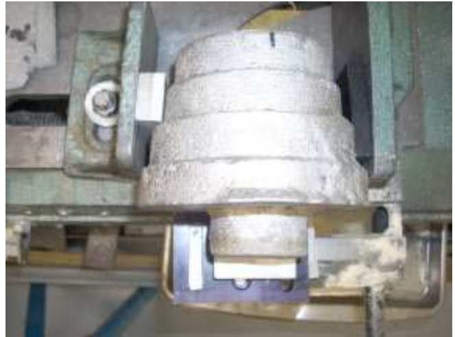
Mounting on Hacksaw Photo by R. G. Sparber
