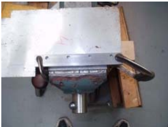
Jig for Cutting Shims
