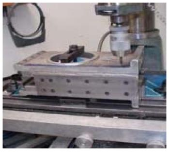
Center Drilling Casting Photo by R. G. Sparber
