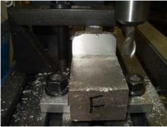
Finished Vertical of Pocket Photo by R. G. Sparber
