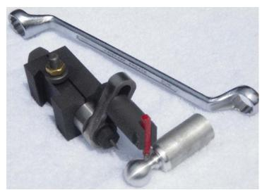
bolts, washers, threaded rod, setscrews, an E-clip, and an O-ring. If you already have a 1" Aloris style boring bar holder, you need only make 4 parts: Shaft, Spacer, Swing Arm, and Tool Bit Holder. Details for machining those parts are shown in the drawings below.
