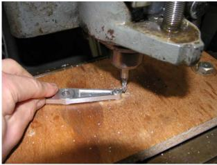
Here's another, similar approach to this job, done on a small brass part. In this case, I used a disk sander rather than an endmill. Brass has a habit of grabbing during cutting, but a disk sander doesn't pull tangentially, so has no tendency to grab. This part was extremely small, so a long rod was bolted to the end to give smoother feed and good control.
