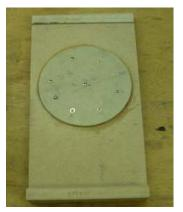
Above is the pattern before I cut the hole. One lesson learned is to write lots of instructions on the pieces to be glued together. The draft is only 1 to 5 degrees and it is easy to stick a piece of wood on upside down. It also prevents me from using a finished strip of wood as a glue spreader.
