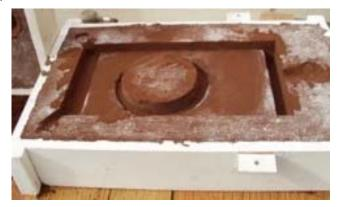
Here you can see the sprue on the right cut into the heaviest part of the pattern void. On the left are my two risers. When metal shows up in these riser holes, I know my void is full. The sprue and riser forms were not pulled out at this time.
