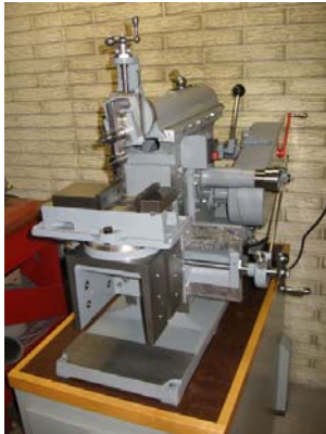
Shaper with Milling Vise Photo by Ron Shimom
