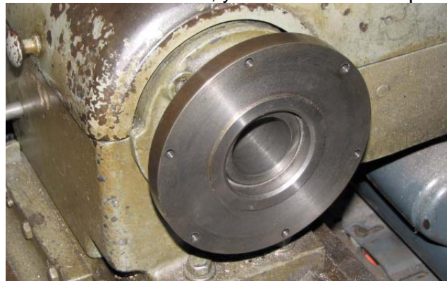
With the chuck off, you see a bare backplate.
