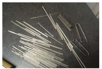
Some small commercial laps that range in size from .045" to .187" diameter. Handy for sizing small bearings. The steel clamps to the right are used to wedge open the splits in the laps.
