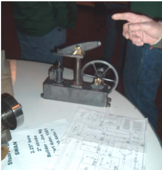
A young man named Adam brought in this Stuart beam engine underway. The well-polished castings and the use of B.A. fasteners caught my attention.
