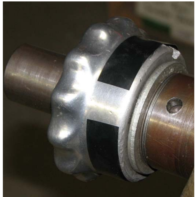
Using Electrical Tape on a Shiny Shaft
