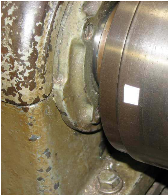
A Patch of Reflective Tape on a Lathe Chuck
