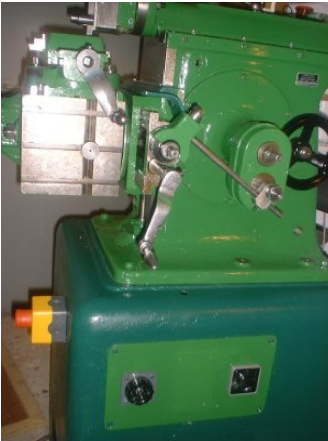
VFD on Front Plate Photo by Siegfried Schmidt
