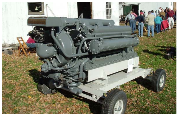
Cal Pixley's Packard V12 PT boat engine (around 2900 pounds!) #1724
