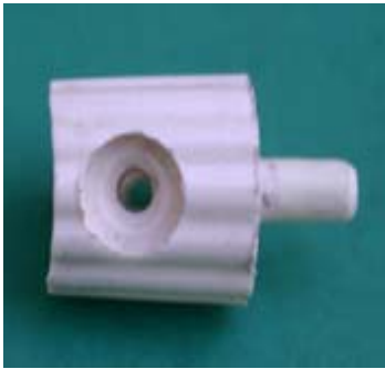
Here, drilled through using a # 45 bit. Yours may be different.
