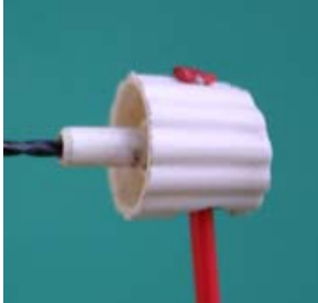
In this case a #23 drill bored through the spray tube (just through one side!)
