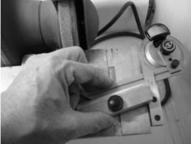
Setting Miter Gage to 14 Degrees
