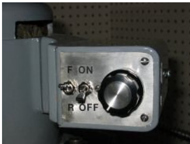
VFD Controls photo by Kay Fisher
