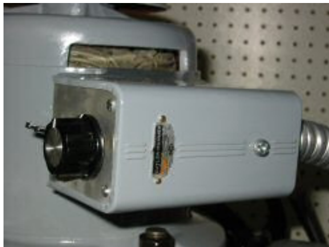
VFD Control Box photo by Kay Fisher
