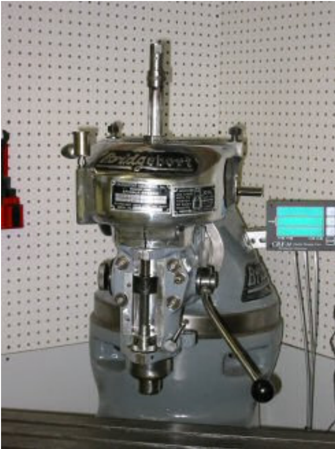
Belt Guard Installed photo by Kay Fisher
