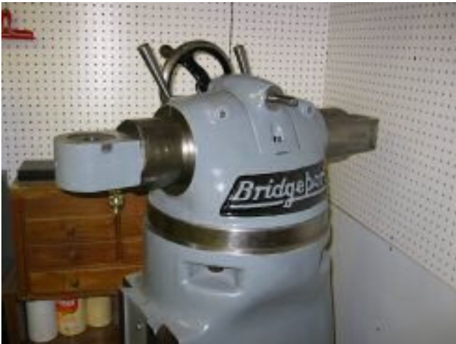
Turret and Ram Installed photo by Kay Fisher
