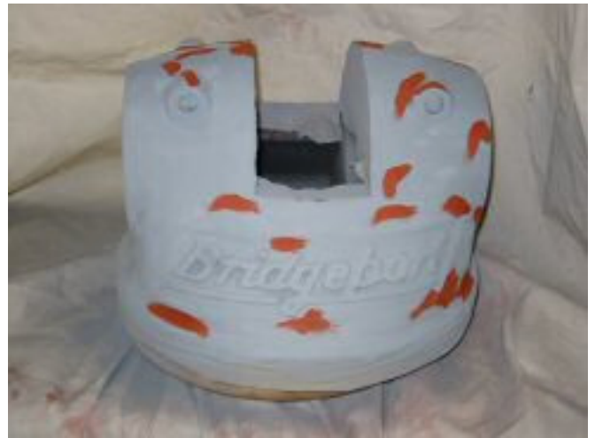
Turret After Glazing Putty 2 photo by Kay Fisher
