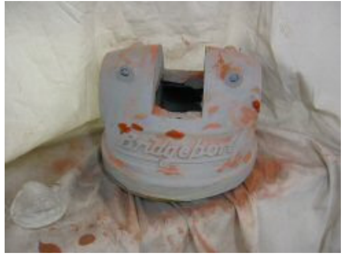
Turret After Glazing Putty photo by Kay Fisher
