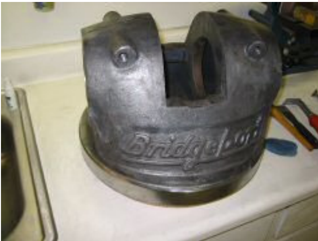
Turret After Wire Brushing photo by Kay Fisher
