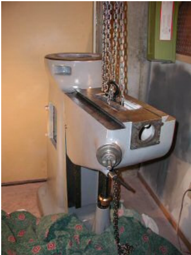
Knee being Installed
