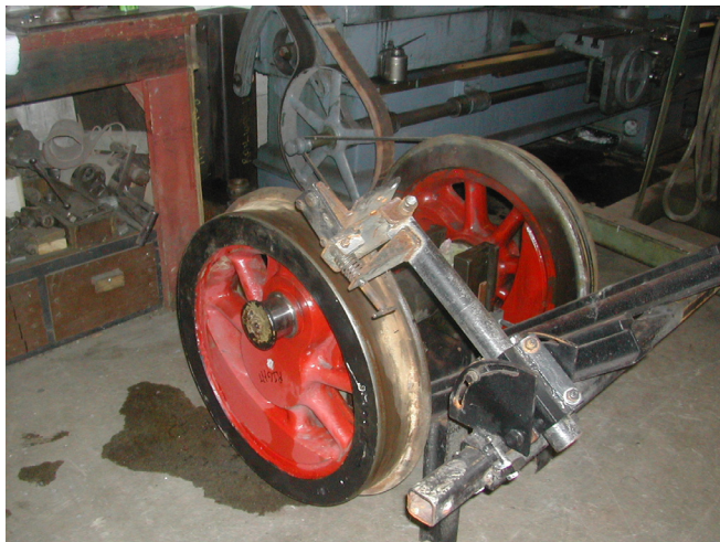
Wheel Tread Beading device
