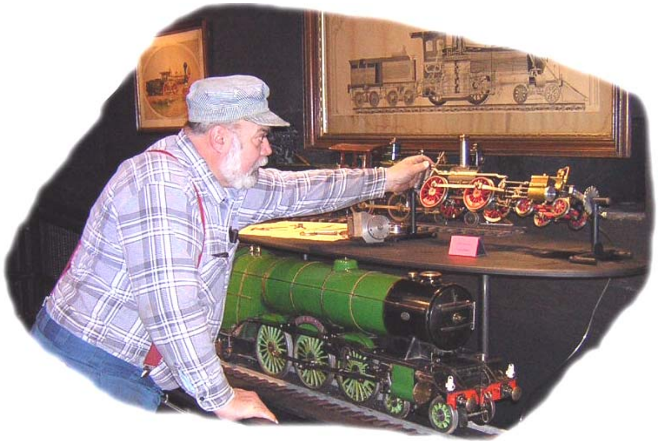
↑ Dick Boucher reaches over the late Walter Bush's "Flying Scotsman" to adjust the cutoff on his 3 1/2" gauge "Virginia" chassis. A completed "Virginia", also built by Walter Bush, sits in the background. Like Todd's engine, the chassis is connected to an air-line. Having it suspended in air makes it easy for spectators to view the valve gear. The locomotive print hanging on the wall is a nice touch!
