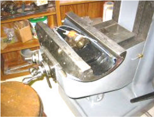
Lube fitting visible on Knee right side Photo by Kay Fisher
