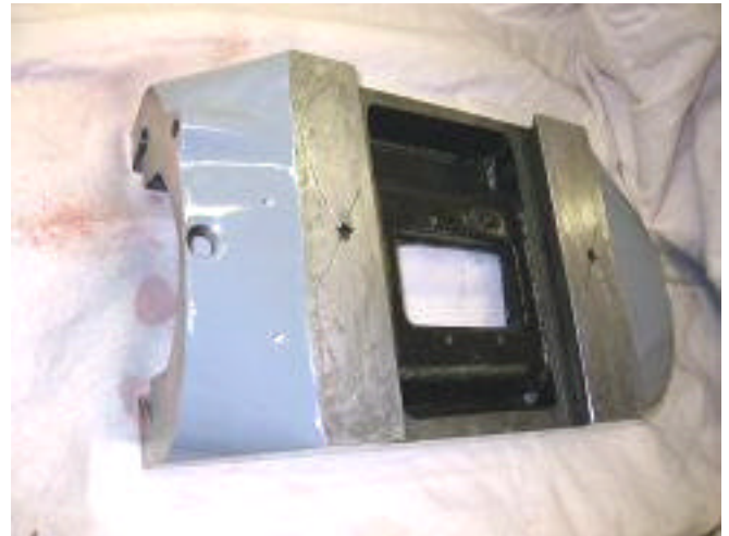
Saddle with Holes Drilled
