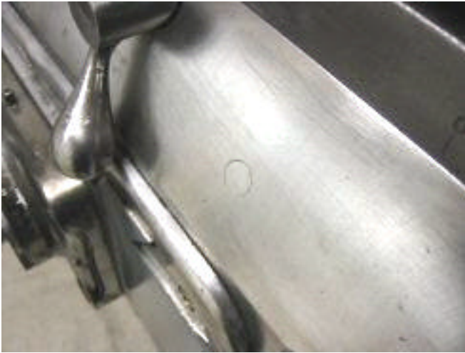
Plug After Filing Down
