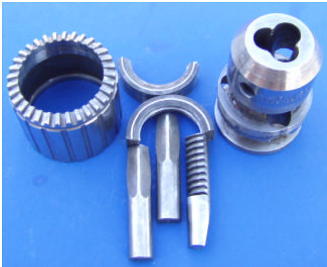
Disassembled Jacobs chuck Bob Beecroft photo
