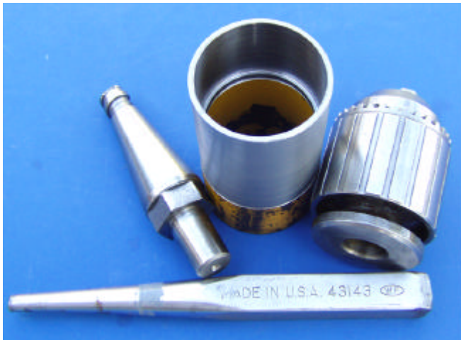
Jacobs chuck, Moore taper, and the tools to disassemble the chuck Bob Beecroft photo
