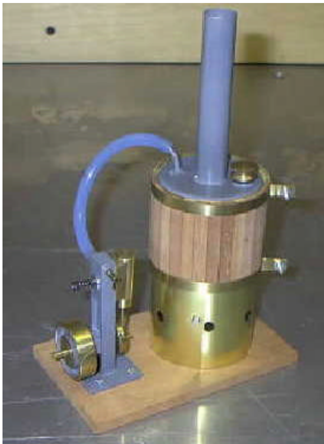
Boiler and Steam engine
