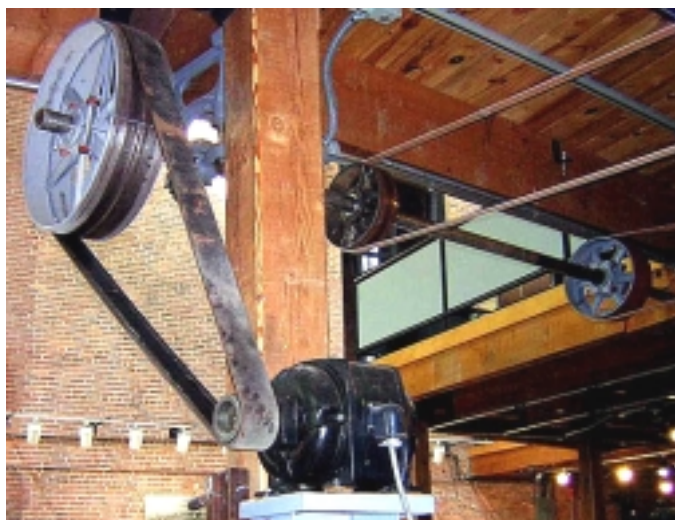
CRMI shafting. Note reduction between electric motor and drive shaft. Power wheels for both shaper and planer are visible.
