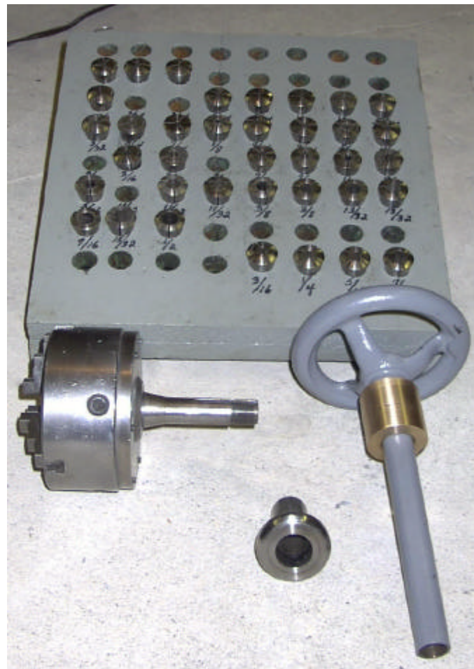
The completed collet closer assembly and all of the parts that make it work
