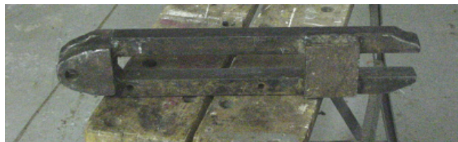
Damaged Ram Lever photo by Pete Verbree
