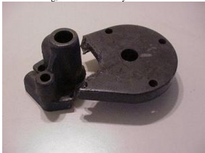
Cracked Clutch Housing photo By Pete Verbree
